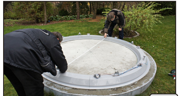
Measuring the inner diameter of the base ring at several positions
