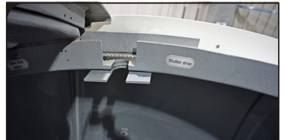
Place where the main shutter engine bracket should be mounted
