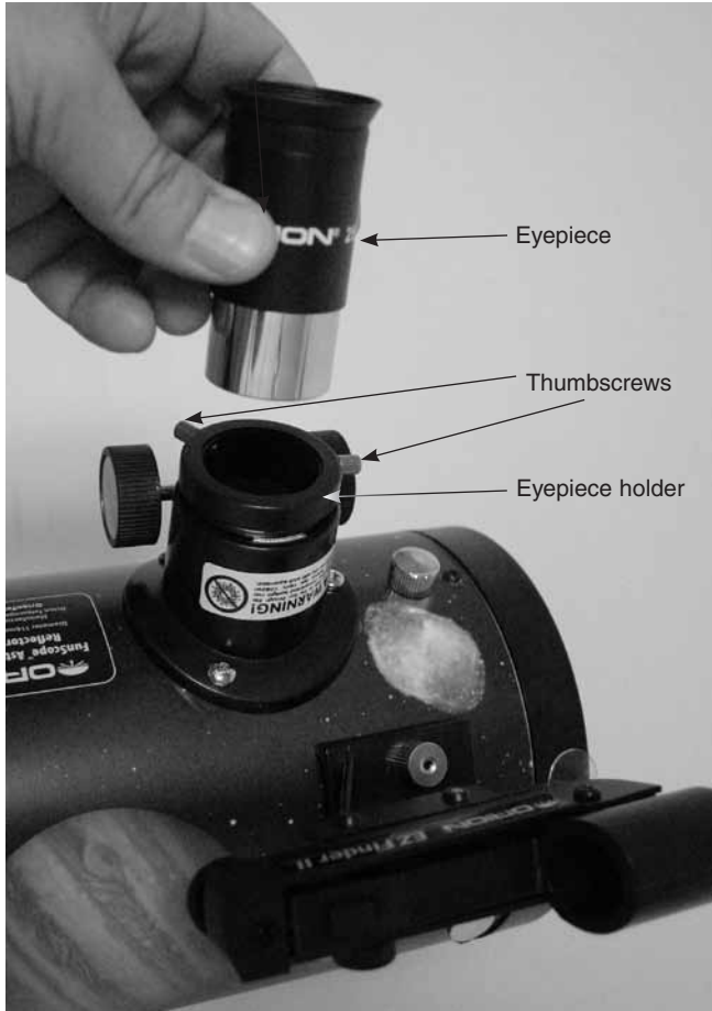
Figure 6. After removing the dust cap on the focuser, insert a 1.25" eyepiece into the eyepiece holder, then lightly tighten the two thumbscrews to secure it in place.
