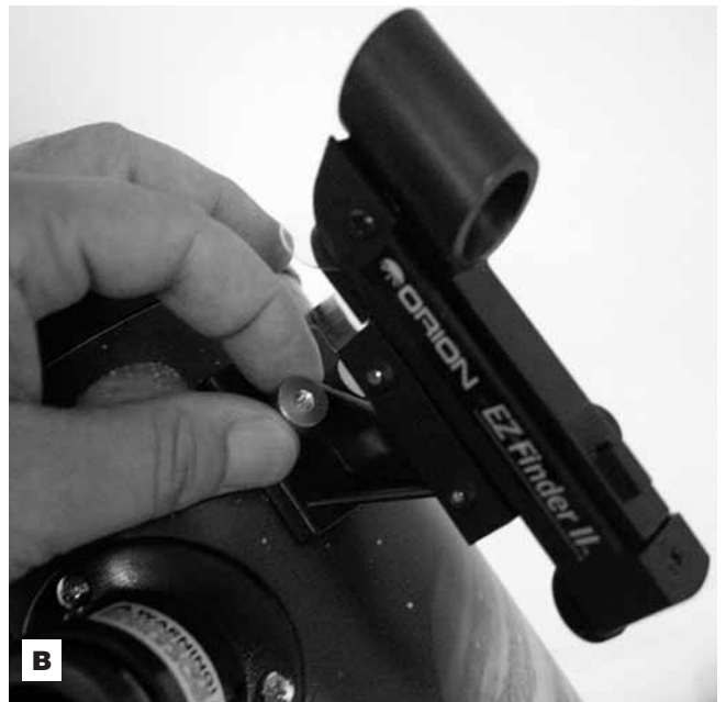
Figure 5. To attach the EZ Finder II, A ) first remove the two thumbnuts near the focuser, then B ) install the EZ Finder II bracket over the two exposed screws, then replace the thumbnuts.
