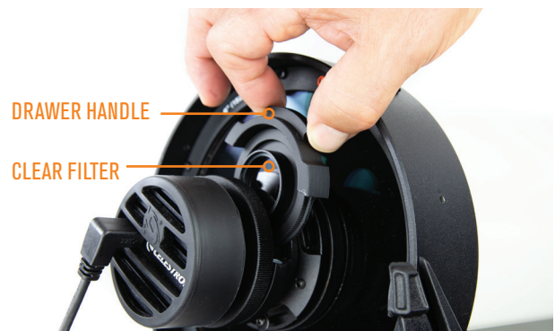
Fig. 15: Grasp the drawer's handle with your fingers and pull outwards to release it from its magnets.
