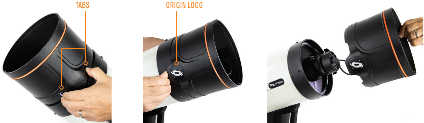
Fig. 13: Remove the lens shade by pressing down on the two tabs with one hand while pushing upward under the Origin logo.
