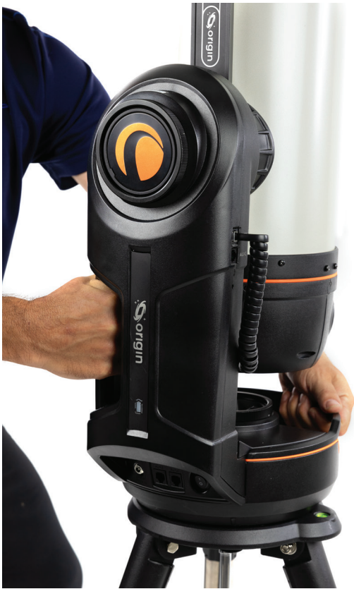
FIG 31: Use the handles on the fork arm and mount to lift Origin.
