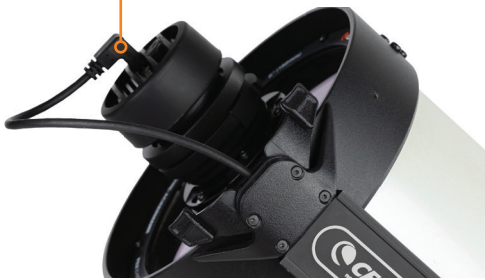
FIG 36: One end of the camera cable plugs into the camera. The other end plugs into one of Origin's USB ports.
