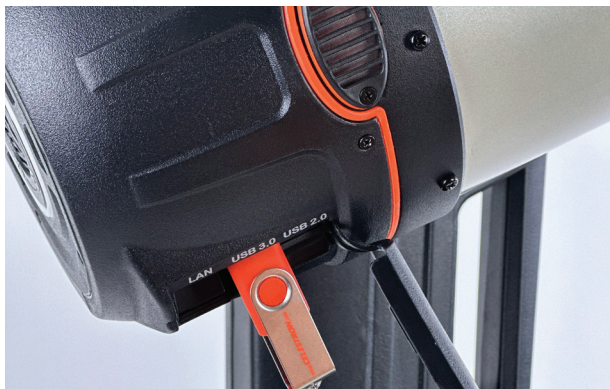
FIG 27: Insert a USB thumb drive into the USB port on Origin's tube to transfer the raw image files.
